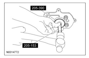
5. Install the axle shaft. For additional information, refer to <a href="Axle Shaft">Axle Shaft</a> in this section.
